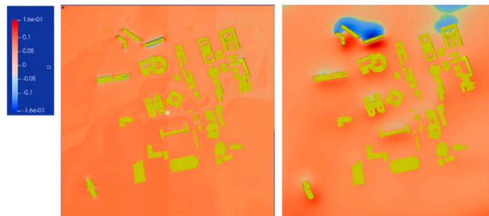
Figure 6. Numerical predictions of the flow field at University of León campus showing the different flow patterns for two different wind directions.
