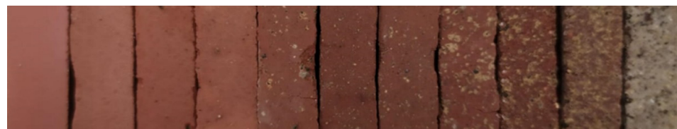
Figure 8. Image of the ceramics conformed with various percentages of clay and contaminated soil. From left to right, CS0, CS1, CS2, CS3, CS4, CS5, CS6, CS7, CS8, CS9 and CS10.
