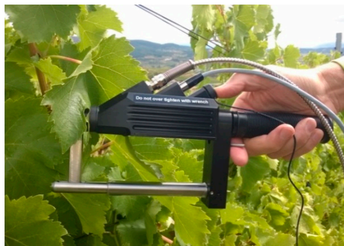
Figure 4. Spectral data collection using a plant probe and leaf clip accessories.
