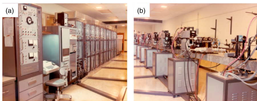
Figure 4. The Battelle Compagnie Générale Electric (CGE) VD-640 Q-switched laser: a) capacitor banks; b) laser rod amplifier. Reproduced with permission. [41] Copyright 2019, MDPI.
