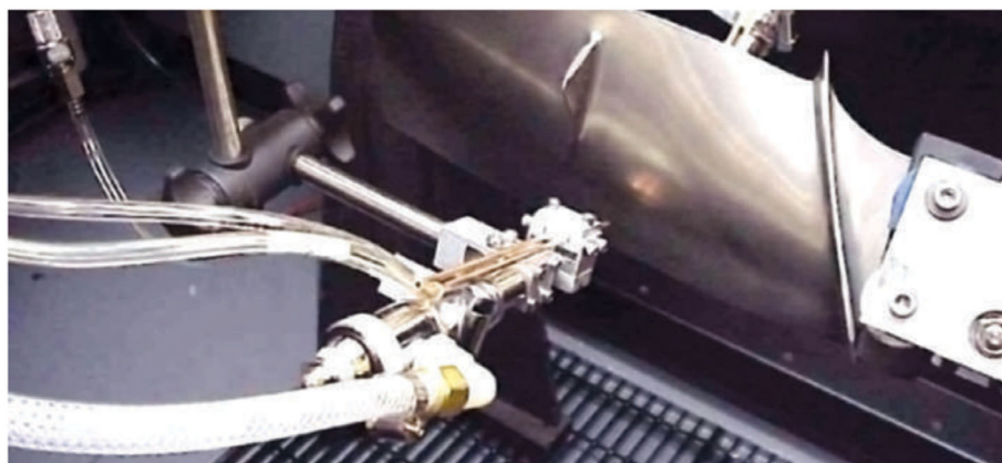
Figure 9. LSP Technologies' Rapid Coater system is positioned for processing an F101 engine blade. Reproduced with permission. [233] Copyright 2009, Springer Nature.
