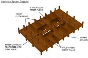
Figure C.1: 'AB-Timber' Structural System Diagram
