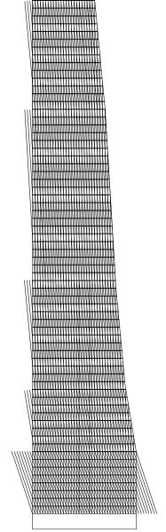
This Diagram Helps to draw attention to system implemented for the 5' grid that both the mullions and diagrid work on - which is between the 20' structural column grid.
