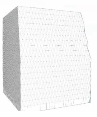
Image Above: (from the development phase of the project) Helps to articulate the importance of the uniformity of the Diagrid to the rest of the structure and how unaligned columns can become an eyesore on the exterior of the building.
