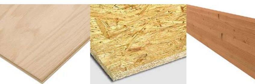
Plywood is a structural panel of Oriented veneer on each level, the panel is strength in both directions. able to gain strength and stiffness in both directions.
