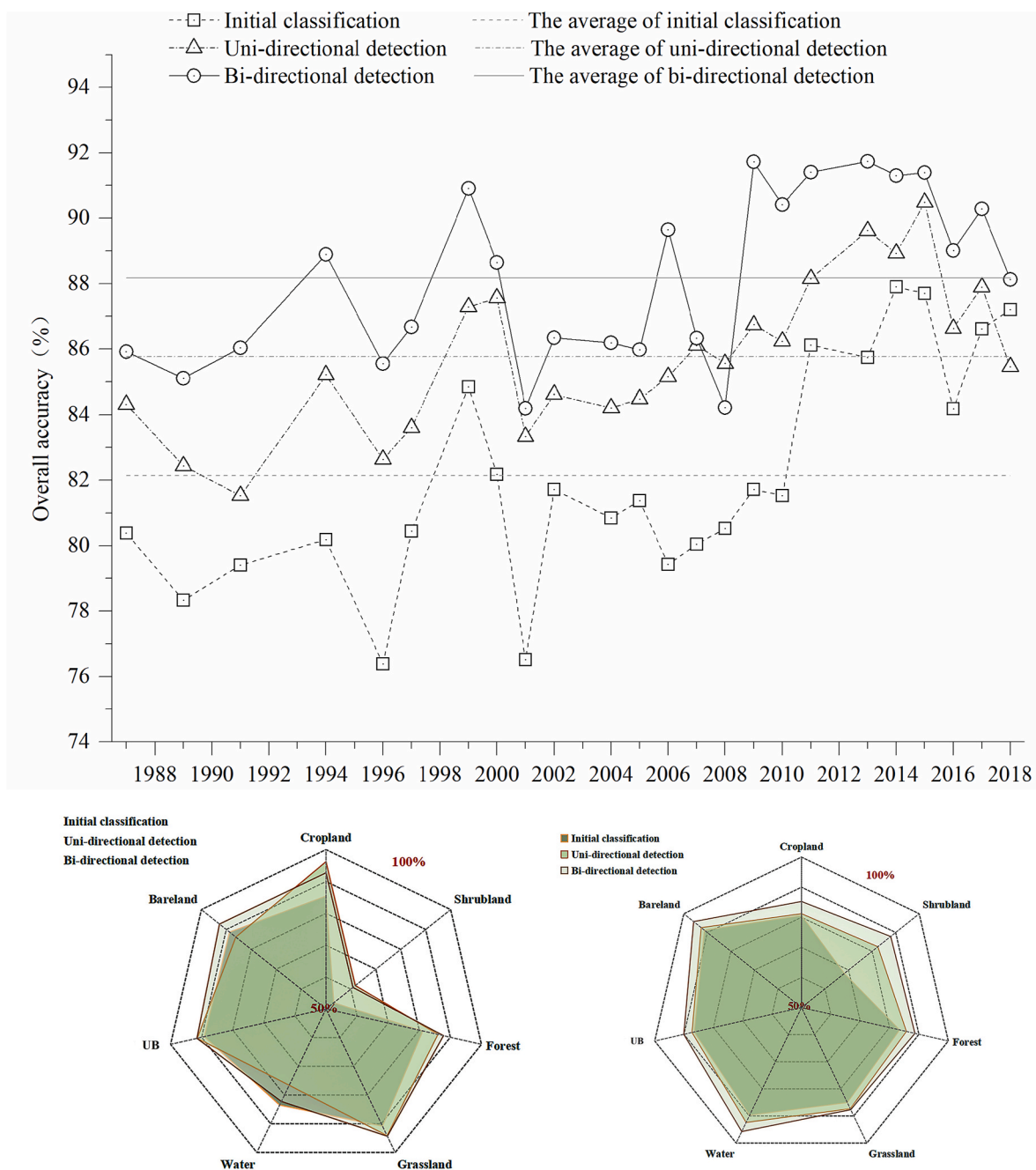
Fig. 7. Accuracy comparison of initial classification, uni-directional method and bi-directional method; (a) overall accuracy; (b) completeness accuracy; (c) correctness accuracy.
