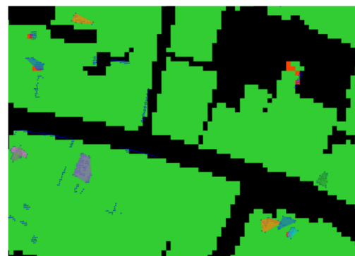
Figure 3. Automatic error detection. The green pixels are the modeled area; the orange pixels are the no-data pixels. The dots are the outlier points, and the translucent polygons indicate larger erroneous areas.
