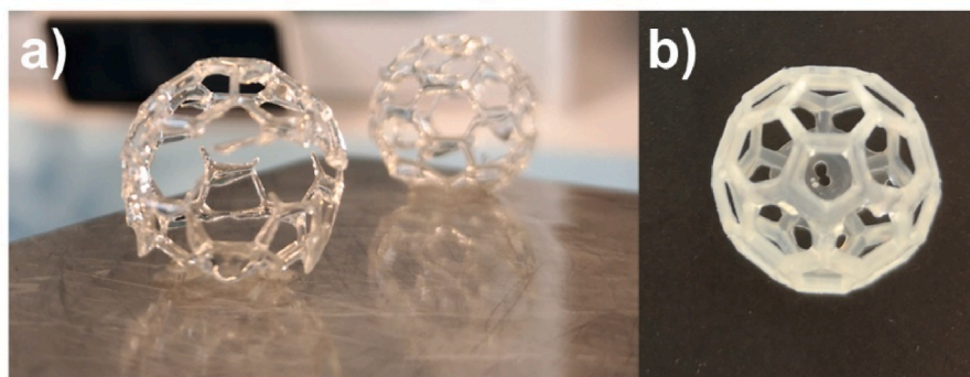
Fig. 8. Photos of the 3D printed fullerene buckyballs at 8 s of the irradiation time using: a) pure polyPEGDA and b) polyPEGDA composition with 6.0% w/v nanosilica. The size of structures is 32 mm.
