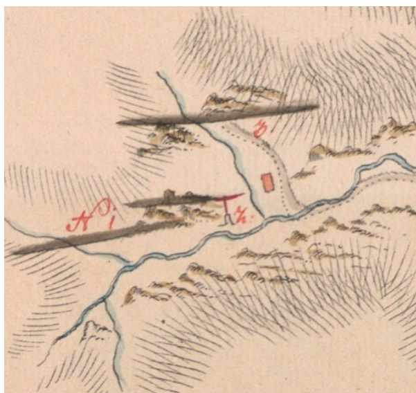
Figure 18. Surface prospecting cuts (1,3) and a tunnel, named Steccaia (2). Figura 18. Rafas (1,3) y un túnel llamado Steccaia (2).
