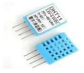
The DHT sensor in Figure 1 is a sensor that can measure air temperature and humidity. The working principle of DHT11 is like an NTC (Negative Temperature Coefficient) thermistor which utilizes changes in resistance when the temperature changes. The working principle of the DHT11 air humidity measurement is like the working principle of a capacitive sensor that utilizes changes in capacitance when there is a change in air humidity.
