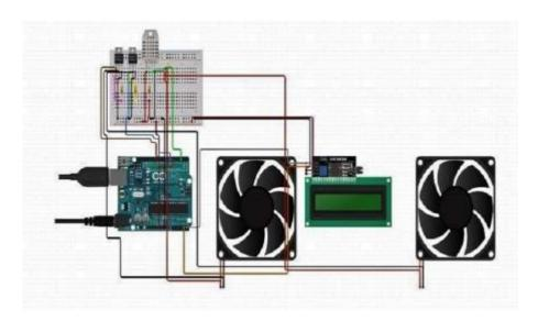
Figure 6 Temperature Control System Design
