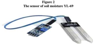
The YL-69 soil moisture sensor is an ideal sensor for monitoring city gardens or water levels in garden plants. This sensor consists of two probes for passing electric current in the soil as shown in
