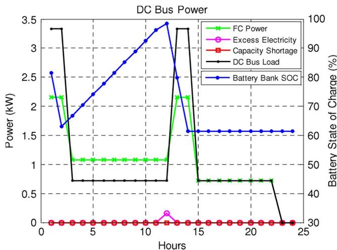
Fig. 9. Simulation of 2.4-kW fuel cell + 12 × 55-A · h batteries in scenario I.
