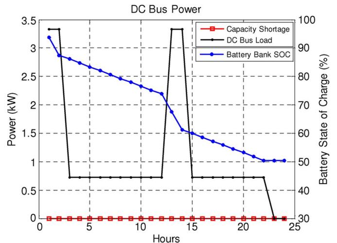
Fig. 10. Simulation of 100 × 55-A · h batteries in scenario I.
