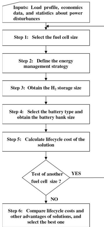
Fig. 3. Algorithm for sizing the backup fuel-cell/battery hybrid power system.
