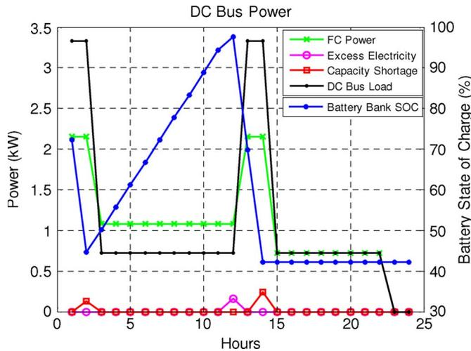
Fig. 8. Simulation of 2.4-kW fuel cell + 8 × 55-A · h batteries in scenario I.
