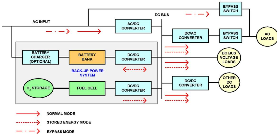
Fig. 2. UPS system configuration.
