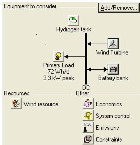
Fig. 4. System configuration entered in HOMER.
