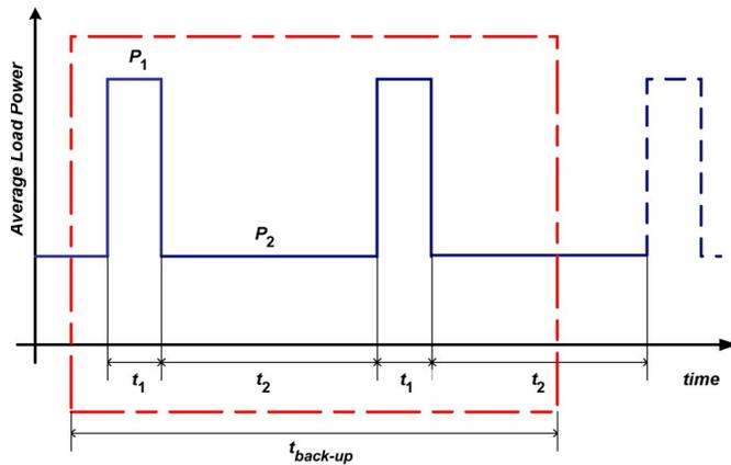
Fig. 5. Typical telecommunication system load.
