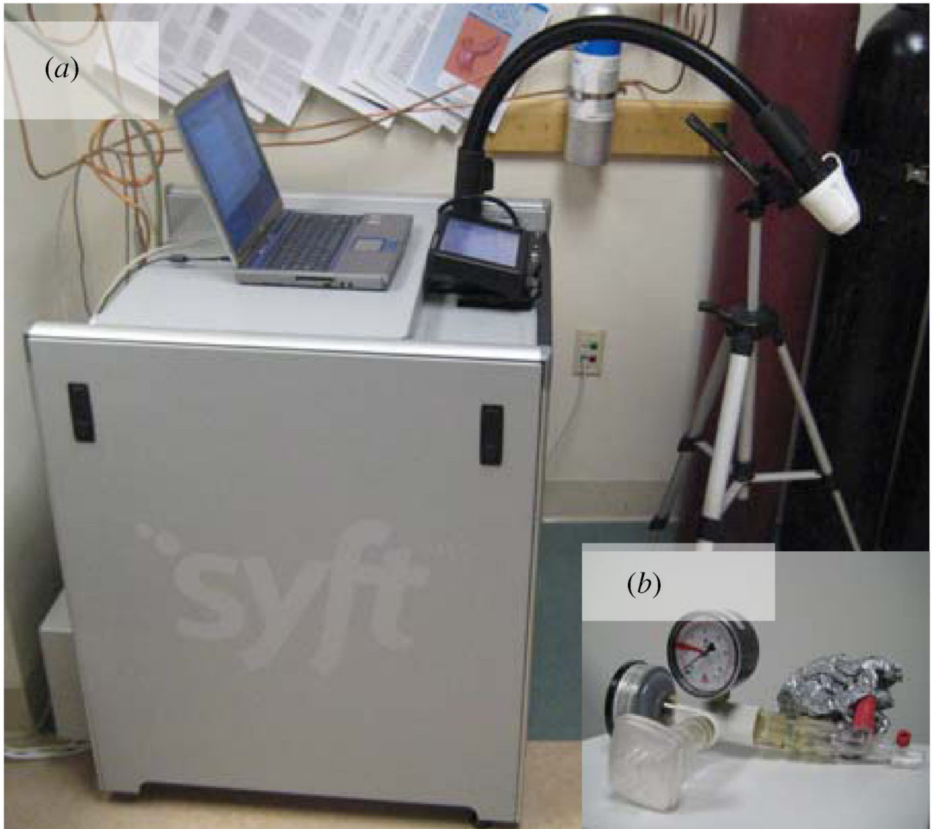
Figure 1. (a) SIFT-MS instrument. (b) Exhaled breath collection device consisting of an air filter, flow meter, mouth filter and breath collection bag. Reproduced with permission from Syft Technologies.
