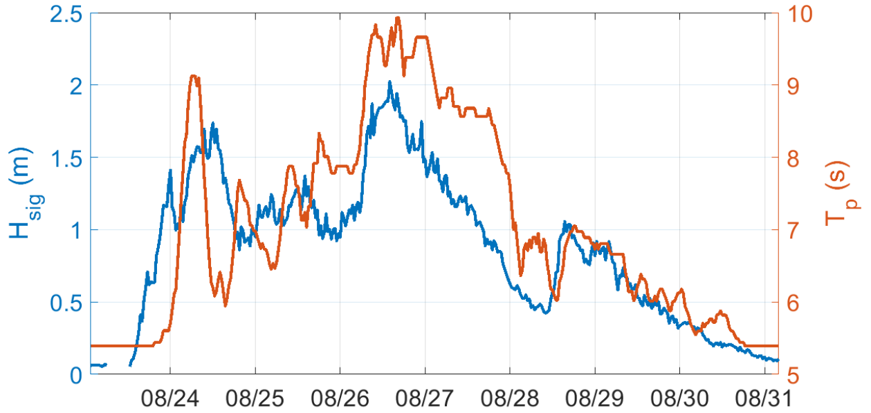
Figure 1.4: ERA5 wave hindcast wave parameters (Hersbach et al., 2018), significant wave height ( H_s ) and peak wave period ( T_p ), for a storm occurring near the Flaxman Island, AK shelf section between August 23 rd and 31 st , 2020. This represents a typical ABS storm and was implemented on modelled output shelf profiles.
