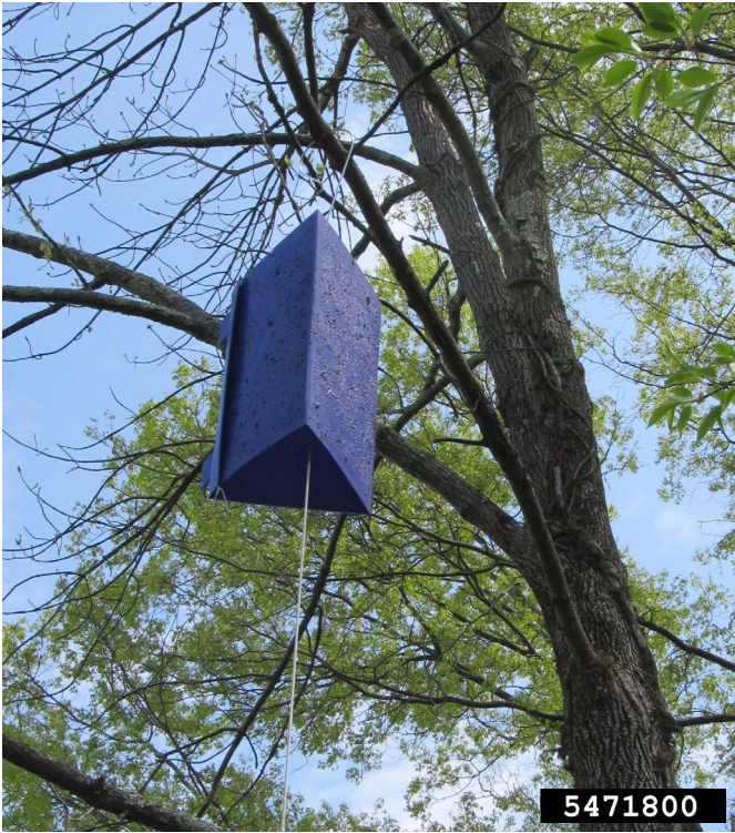
Figure 31. A three-sided purple prism trap hanging vertically in an ash tree. Photo: K.R. Law, USDA APHIS PPQ, Bugwood.org.
