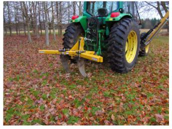
**Figure 5.4.** This tractor is equipped with double shanks 18 inches (46 cm) apart to create offset rows where the poplars are planted 9 inches (23 cm) off the row center. Photo: N. Haider.
