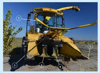
**Figure 11.1.** Parts of the New Holland 130FB Coppice Header. Photo: N. Haider.
