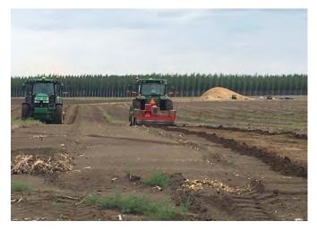
Figure 13.6. A subsurface mulcher breaks up and incorporates the woody debris into the soil. Photo: A. Himes.
