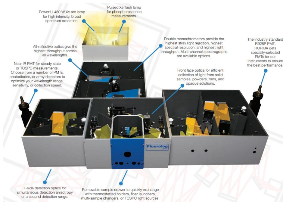
Fig. 2.11. Schematic of Horiba Fluorolog spectrometer. The image is from the Fluorolog Brochure 26 .
