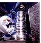
**Lithographic lenses:** By example, a figure of a Zeiss Starlith lens, usable for creating masks with 100 nm structures. It has a maximum aperture of f/0.45 for a wavelength of 193 nm (source: http://www.zeiss.de/de/semicon/home.nsf/Inhalt-Fra-
