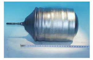
Figure #14: Freiberger GaAs crystal (source: http://www.fcm-germany.com/).
