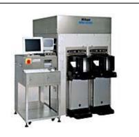
**Measurement equipment:** By example, a Nikon measurement system for checking exposures. Measures mask images with a lowaberration optics and achieves a precision of 2 nm, about the size of the molecules (source: Nikon 2002b).
