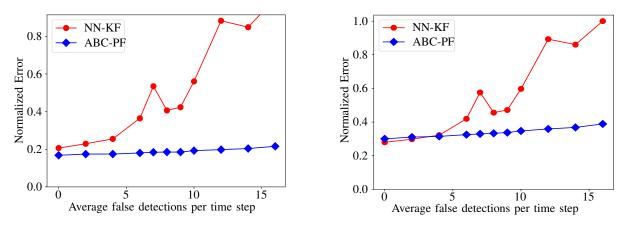
Fig. 2: Errors for different values of  $\lambda$ , averaged over the whole trajectory and 100 runs. Left: OSPA of means, see (8). Right: MMOSPA between ground truth and particles, see (9).
