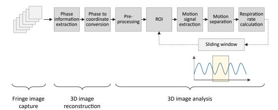
**Figure 1.** Overview of the developed system from capturing data to the extraction of the respiratory parameters.
