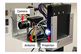
Figure 2. Setup of the 3D sensor prototype.
