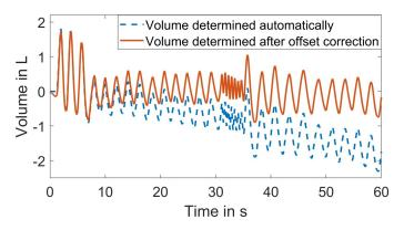
Figure 6. Comparison of the volume signal before and after baseline correction.
