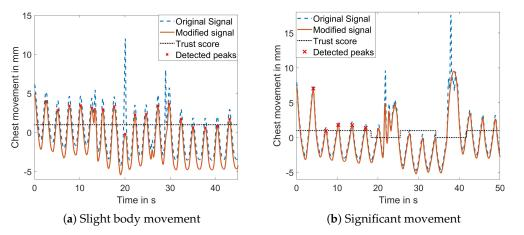
**Figure 9.** Result of the motion separation algorithm and the introduced binary trust status with different levels of body movements.
