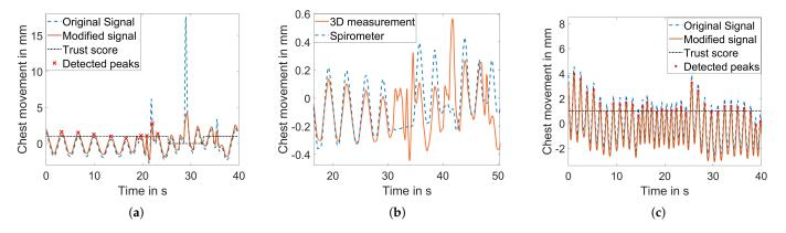
**Figure 10.** Result of the motion separation algorithm for three different breathing patterns and subject behavior. (a) Shallow breathing with slight body movement. (b) Holding the breath with body movement. (c) Fast breathing.
