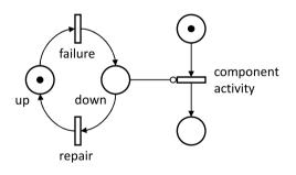
Fig. 7. Failure model of a system component.
