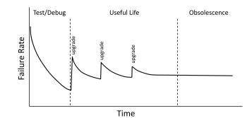
Fig. 3. Revised bathtub curve for software reliability [12].
