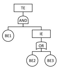
Fig. 6. Fault tree with top (TE), intermediate (IE) and basic events (BE).
