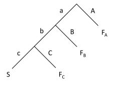
Fig. 9. Structure of a THERP event tree.
