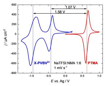
Figure 2. Cyclic voltammograms of X-PVBV $^{2+}$ - (blue) and PTMA- (red) based composite electrodes in half-cells vs. Ag pseudo-reference electrode with the DES NaTFSI:NMA in its eutectic molar ratio 1:6 as electrolyte at a scan rate of 1 mV s $^{-1}$ .
