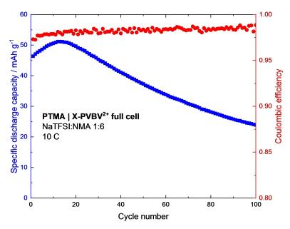
Figure 4. Galvanostatic charge-discharge cycling of the X-PVBV<sup>2+</sup> | PTMA full cell with the DES NaTFSI:NMA in its eutectic molar ratio 1:6 as electrolyte at a rate of 10 C showing the specific discharge capacity (blue) and the Coulombic efficiency (red) for 100 cycles.
