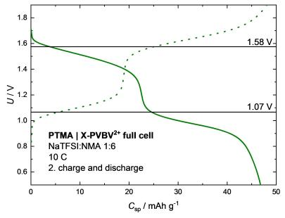
Figure 3. Voltage profile for the second galvanostatic charge (dashed line) and discharge (solid line) of the X-PVBV<sup>2+</sup> | PTMA full cell with the DES NaTFSI:NMA in its eutectic molar ratio 1:6 as electrolyte at a rate of 10 C. The black lines indicate the potential differences between the redox events of PTMA and X-PVBV<sup>2+</sup> extracted from cyclic voltammetry (Figure 2).
