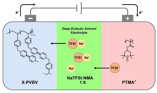
Figure 1. Schematic figure of the charged all-organic battery composed of the DES NaTFSI:NMA 1:6 as electrolyte, PTMA as active material in the positive electrode and X-PVBV<sup>2+</sup> as active material in the negative electrode. Electron and ion movement indicates the discharge process.
