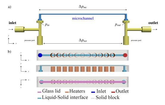
Figure 5: Numerical domain schematics: a) isothermal simulation for simpleFoam b) diabatic simulation for chtMulti-RegionFoam
