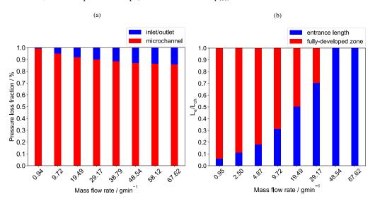
Figure 10: (a) Contribution of the inlet and outlet pressure loss ( $p_{in} + p_{out}$ , blue area) and the microchannel pressure drop ( $p_{mc}$ , red area) to the total experimentally measured pressure  $\Delta p_{tot}$ ; (b) Ratio of entrance length to the microchannel length based on numerical simulation
