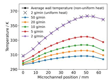
Figure 18: Numerical simulated average microchannel wall temperatures for non-uniform heat source assumption and at  $2 \text{ g min}^{-1}$  additionally for uniform heat source assumption
