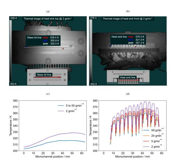
Figure 17: Thermal images at 2 g min<sup>-1</sup> of the heat sink top with glass lid (a), of the heat sink front (b) with line markings of the respective temperature line profiles along the glass lid outside from the microchannel inlet to outlet (c) and along the heat sink front from the first cartridge heater to the last cartridge heater (d)
