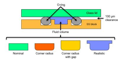
Figure 6: Numerical abstraction of the cross-sectional area (respectively fluid volume) of the experimental microchannel with increasing consideration of geometric details from left (nominal) to right (realistic). The third cross-sectional shape colored in yellow is utilized in the final numerical simulation.
