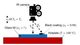
Figure 4: Schematic of Pyrex glass emissivity measurement procedure using a thermal imaging camera (IR camera). The emissivity  $\epsilon_2$  of the glass lid is determined by measuring the temperature  $T_1$  of the glass lid with a black coating with a known emissivity  $\epsilon_1$  and by matching the temperature measurement of the glass lid without black coating immediately adjacent to the coating  $T_2$  by adjusting the emissivity of the camera till  $T_2 = T_1$
