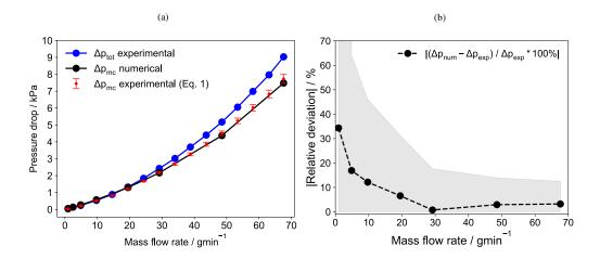
Figure 9: (a) Experimental and numerical pressure drop; (b) Magnitude of the relative deviation =  $100\% \cdot |(\Delta p_{num} - \Delta p_{exp})|$   $\Delta p_{exp}|$  of the pressure drop simulation from the pressure drop calculated with Eq. 1. The gray shaded area marks the uncertainty area  $100\% \cdot |(\Delta p_{num} - \Delta p_{exp} \pm u_{\Delta p_{mc}})|$  linked to the experimental measurement uncertainty  $u_{\Delta p_{mc}}$  calculated with Eq. 36 as given in APPENDIX B.
