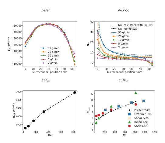
Figure 19: Simulated axial heat flux (a), simulated local Nusselt number compared with Nu(x) (dashed lines) calculated with Equation 16 [44] (b), average heat transfer coefficient (c) and simulated average Nusselt number (d) for mass flow rates between 2 to 49 g/min
