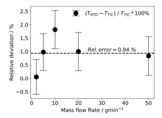
Figure 15: Relative deviation  $(T_{RTD} - T_{T/C})/T_{T/C} \cdot 100 \%$  of the RTD temperature measurement at the outlet of the microchannel from the T/C type measurement of the liquid temperature 18 mm downstream at the heat sink outlet
