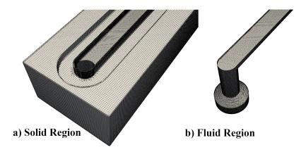
$Figure\ 7:\ A\ sample\ of\ the\ grid\ for\ conjugate\ heat\ transfer\ simulation\ using\ cht MultiRegion Foam$
