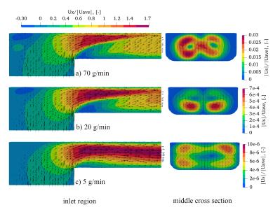
Figure 11: Velocity contour in the  $90^{\circ}$ -bend: (left) the middle plane at the inlet region, (right) the cross-section in the middle of microchannel at x = 32.5 mm
