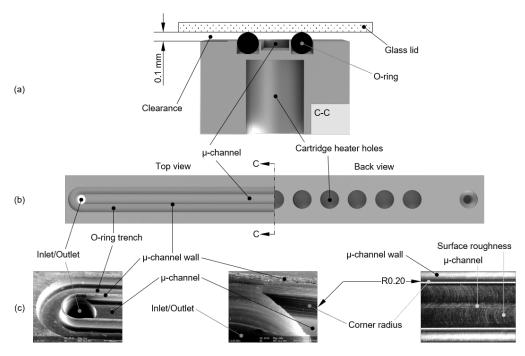
Figure 2: Stainless-steel microchannel: Cross-sectional view (a), top and bottom view (b) and scanning electron microscope images of the inlet with channel wall and surrounding O-ring cavity (left), the corner radius at the inlet (center) and the surface roughness of the channel bottom (right) (c)
