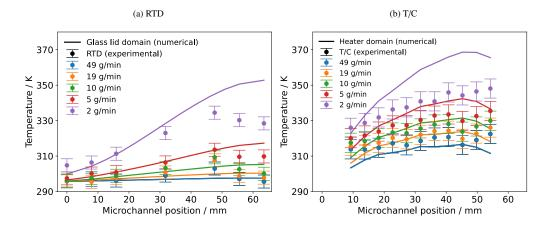
Figure 14: Measured and simulated temperature profiles along the microchannel from the inlet to the outlet: RTD and glass lid domain temperatures (a), T/C and heater domain temperatures (b). Wall temperature is plotted for numerical simulation.
