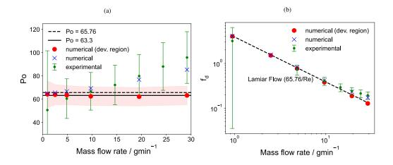
Figure 13: Comparison of (a) Poiseuille number and (b) friction factor from experimental data for the entire microchannel and numerical data computed for the entire microchannel and for the fully-developed region of the microchannel
