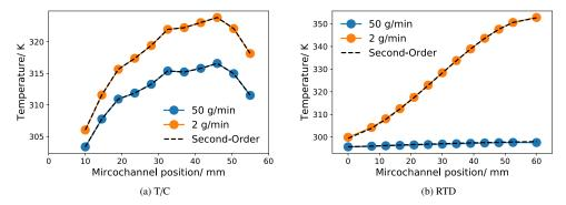
Figure 20: The temperature profile with first-order schemes. The result for second-order simulations is plotted with a black dashed line.
