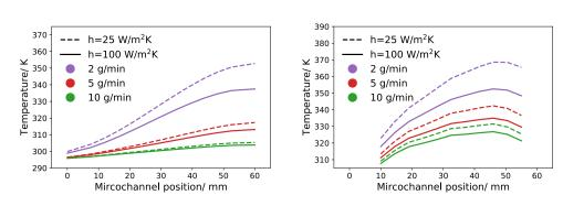
Figure 16: Impact of the chosen heat transfer coefficient h value on the simulated temperature profile
