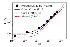
Figure 12: Entrance length of the present numerical study compared with the numerical simulation by Galvis *et al.* [33] and experiments by Ahmad and Hassan [34]. The entrance condition is given in Tab. 3.
