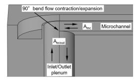
Figure 3: 90° bend causing pressure loss at the microchannel inlet plenum due to flow contraction and pressure recovery at the microchannel outlet plenum due to flow expansion
