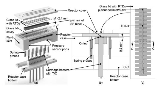
Figure 1: Microchannel setup: exploded view (a), the cross-sectional view (b) and top view on the glass lid with RTDs above the SS microchannel block (c)
