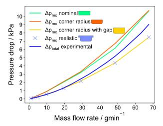
Figure 8: Numerically simulated microchannel pressure drop for the microchannel abstraction levels shown in Fig. 6 together with the experimentally measured pressure drop  $\Delta p_{tot}$
