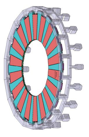
**Figure 1.** Schematic drawing (same comment for other captions) of the installed GE1/1 detectors in staggered arrangement in the CMS experiment [3]. Highlighted in blue (light) are the long detectors and in red (dark) are the short ones. Reproduced from [3]. CC BY 4.0.
