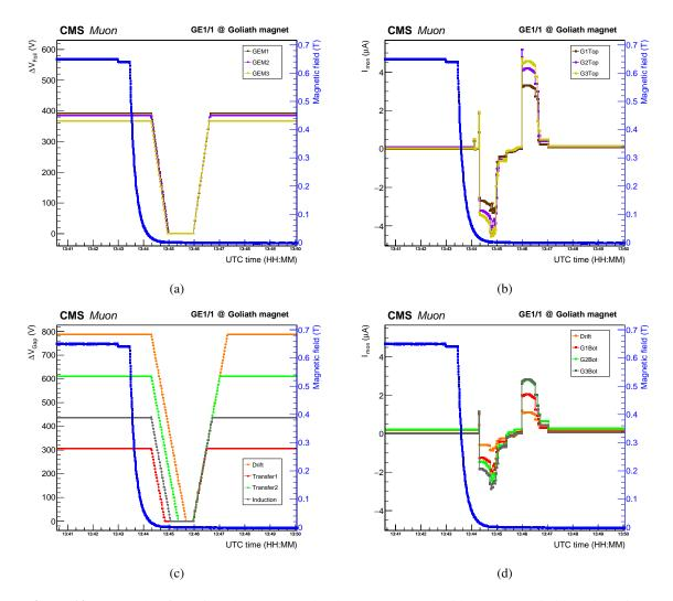
**Figure 10.** Example of monitored currents and voltages, measured with CAEN A1515 board, during a magnet field ramp that caused a discharge and a trip. The four plots show the same discharge event. (a) and (b) show the monitored voltages and currents across the three GEM foils, while (c) and (d) show the same across the GEM gaps. The measured value of the magnetic field is also displayed in each case (blue dots and vertical scale on the right).
