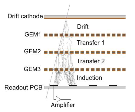
**Figure 2.** Diagram showing the functioning principle of a triple-GEM detector: an avalanche induced by a muon crossing the detector develops from drift, across the three foils, and generates the signal on the readout.
