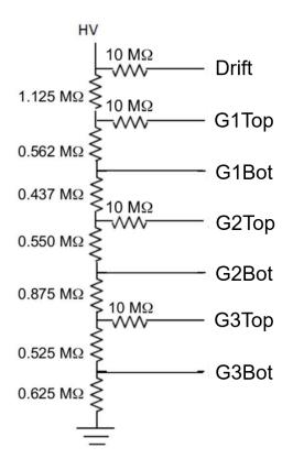
Figure 5. Scheme of the reference resistors [8]. Reproduced with permission from [8].
