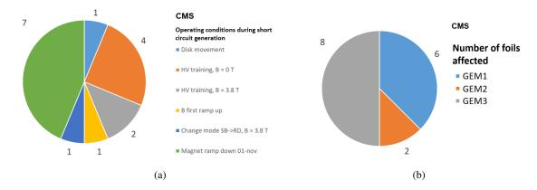
**Figure 8.** (a) Operating conditions at the moment of short circuit creation from the beginning of the GE1/1 commissioning up to the  $5^{\text{th}}$  November 2021; (b) foils affected by short circuit from the beginning of the GE1/1 commissioning up to the same date.
