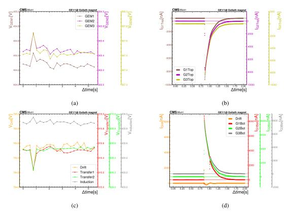
**Figure 11.** Example of discharges observed through pico-ammeter: (a) monitored voltages across the three GEM foils, (b) monitored currents flowing on GEM top electrodes, (c) monitored voltages across the GEM gas gaps, (d) monitored currents flowing on drift and GEM bottom electrodes.
