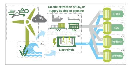
Figure 2. Schematic representation of the offshore PtX process chain, adapted from [25].
