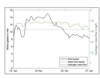
Figure 9. Simulation of hydrogen flow after the  $H_2$  separator based on wind speeds for SEN-1 area.
