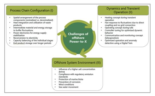
Figure 3. Summarized overview of the challenges of offshore PtX, grouped into the 3 categories presented: process chain configuration (I), dynamics and transient operation (II) and offshore system environment (III).
