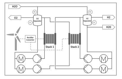
**Figure 8.** Configuration of the simulated electrolysis container with two of the four stacks of the plant coupled with a wind turbine.
