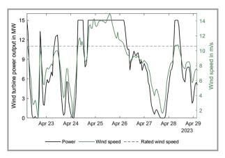
**Figure 7.** Simulated power generation curve based on the IEA 15 MW reference wind turbine in the SEN-1 area. Above the nominal wind speed of the turbine, it outputs almost constant maximum power.
