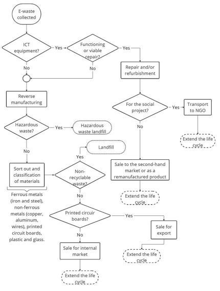
Figure 5. Reverse channels of electrical and electronic equipment in Florianópolis (from collection to reverse manufacturing).
