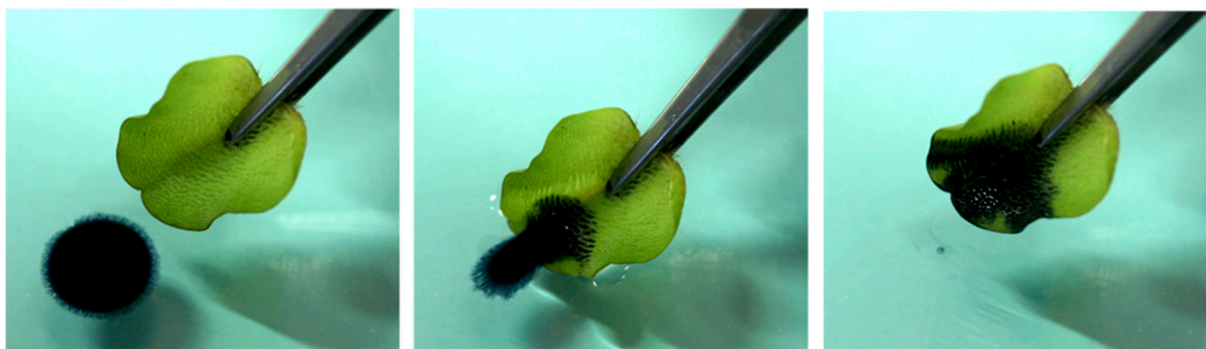
Figure 1. Adsorption and transport of a crude oil droplet from a water surface by a leaf of Salvinia molesta . The oil is adsorbed completely within seconds [8]; see Video S1 in the Supplementary Materials.
