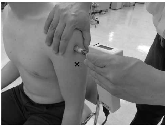
Figure 3. Recording of pressure pain threshold (PPT) on the deltoid muscle. Assessment site was determined as a midpoint between the lateral edge of acromion and the injection site (x).
