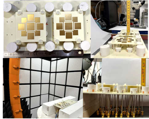
Fig. 18. Prototype of the manufactured subarray
