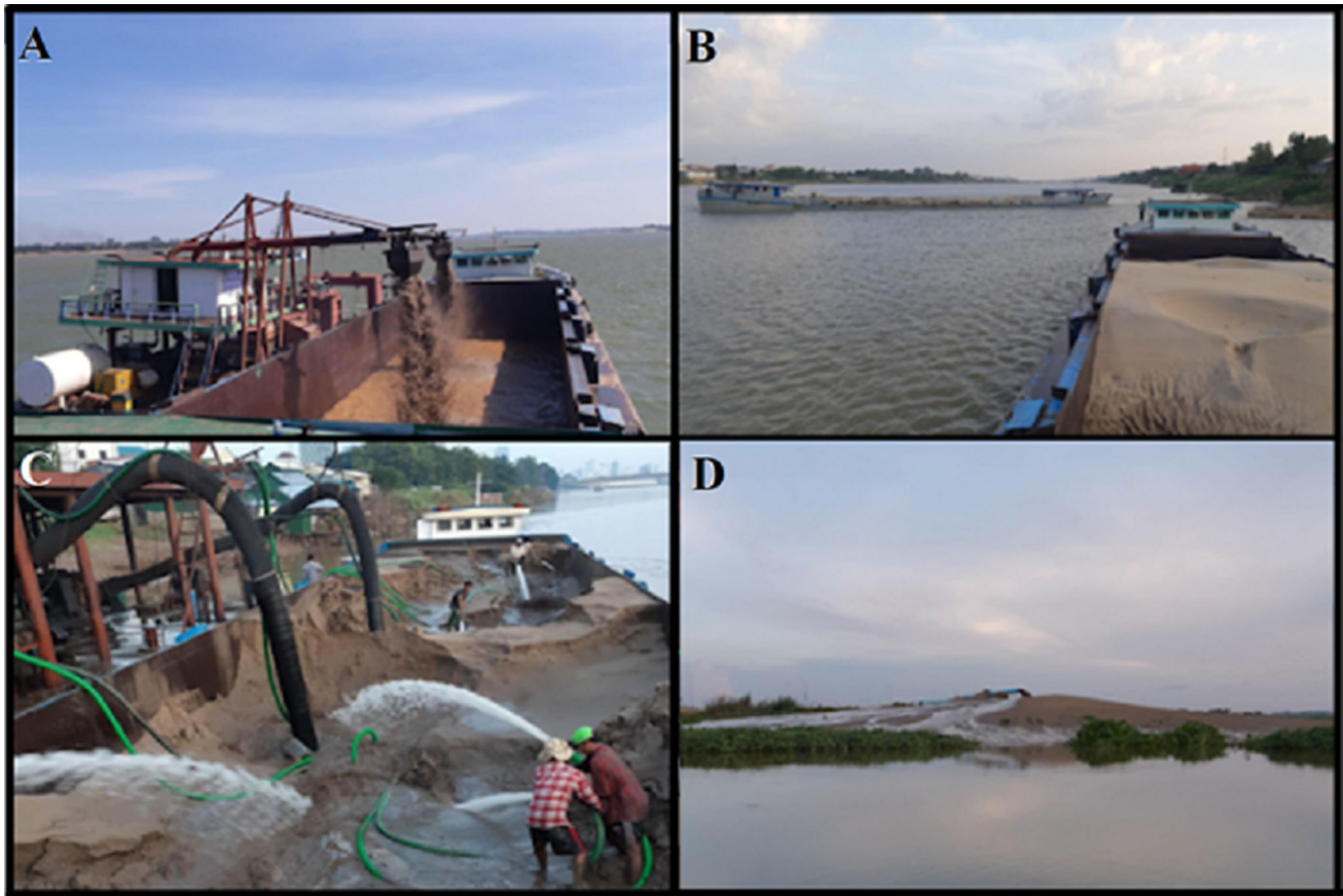
Fig. 3 A Dredging sand in Kampong Cham province. B Transporting sand by barge to Phnom Penh. C Pumpers liquefying sand so it can be pumped onto land. D Wetland south of Phnom Penh filled with sand to prepare land for real estate development. Photos by Lukas Van Arragon
