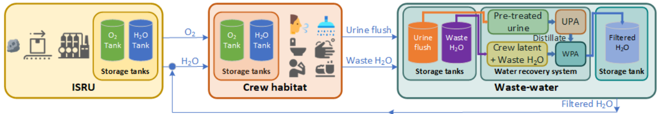
Fig. 1: Three interacting subsystems for maintaining oxygen and water flows in the lunar base (UPA/WPA: urine/wastewater processor assembly)
