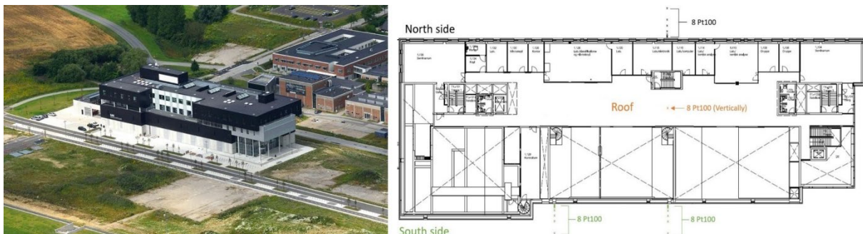
Figure 1. Aerial view of the study case building (left). Blueprint of the study case building with the location of the 4 air temperature measurement setups.
