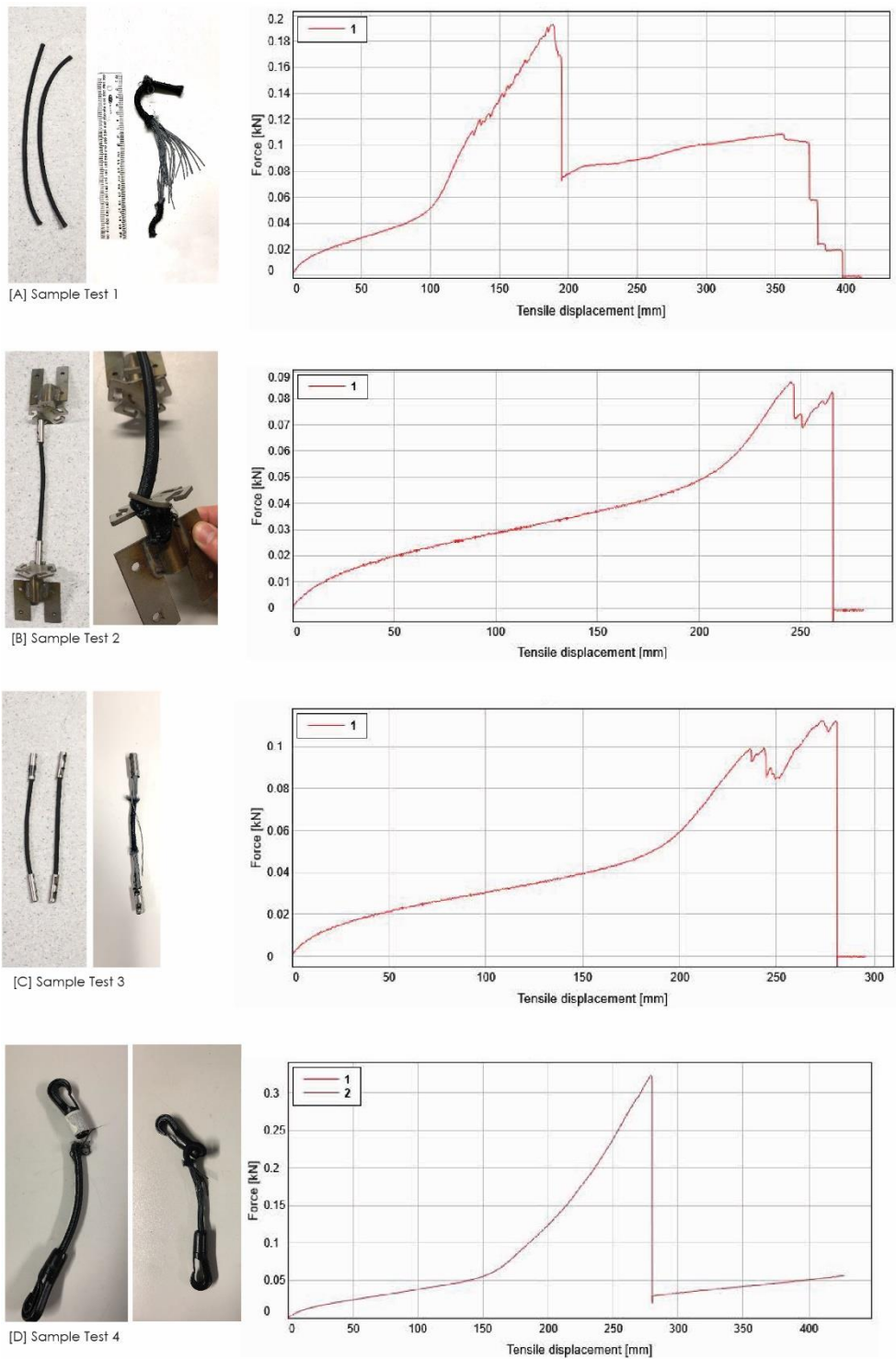
Figure 4. Ultimate Tensile Strength testing of connectors and elastic cords.
