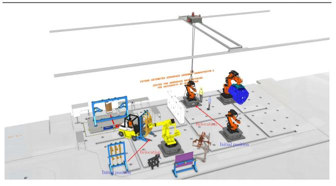
**Fig. 4** Agent relocation for layout reconfiguration. In Omnifactory, there are two main ways to relocate agents. First, agents can be relocated by crane. Second, some small devices can be moved by forklift. Note that, we design reconfigurable grids to position robot and provide pneumatic port and power supply
