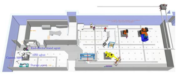
(b) Digital twin of Omnifactory established in Visual Components.
