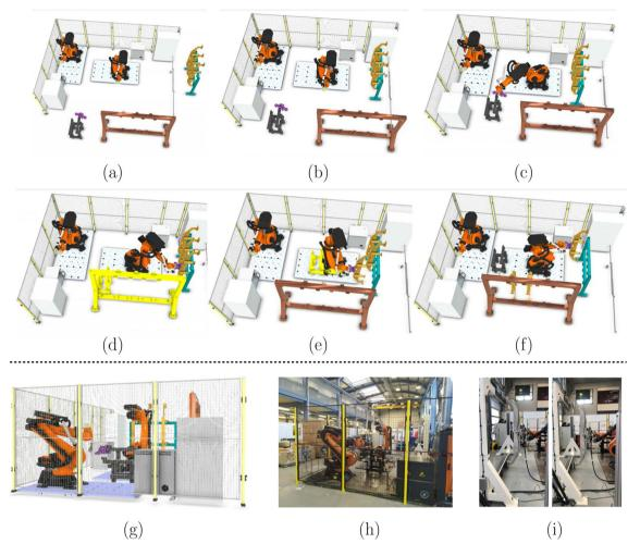
**Fig. 16** Experimental learning result and real-world assembly implementation. The snapshots of the cooperative learning for the assembly work cell are presented from **a** to **f**. In addition, the learned result (dig-
