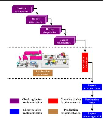
**Fig. 11** Calculating procedures of different fitness functions. Given that two types of interactions introduced in this work, the self-interest fitness functions are checked before the implementation of the production processes. However, since there might be clash during the implementation, the collision is detected throughout the whole implementation. Finally, the layout compactness is calculated after the implementation, along with production time and layout arrangement cost
