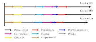
**Fig. 23** Comparison of the elapsed time of the three optimisation schemes. For the three optimisation schemes, the elapsed time for each production process are presented in the above figure. The total time is listed at the end of each optimisation scheme
