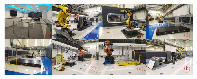
**Fig.2** Omnifactory (Future Automated Aircraft Assembly Demonstrator Phase 2, FA3D2). The Omnifactory is designed as a experimental testbed for digital, informatics enabled, and reconfigurable aerospace
