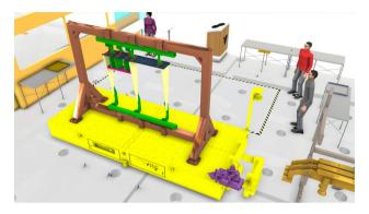
Fig. 8 Collision detection. The collision among different agents is detected during the implementation of the production processes
