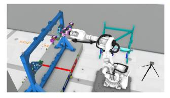
**Fig. 7** Wrist singularity triggered by relocation. The relocation might cause robot wrist singularity. Therefore, it is considered in this work and a fitness function is introduced to avoid this issue
