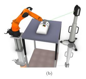
**Fig. 1** Comparison between the 2D projection model and the digital twin model in the layout optimisation. **a** Top view of the metrology cell. **b** The digital twin of the metrology cell. Compared with the top view of the metrology cell which is a 2D projection, the digital twin model could provide more comprehensive information, such as Cartesian scan trajectory, laser tracker motion and other spatial information
