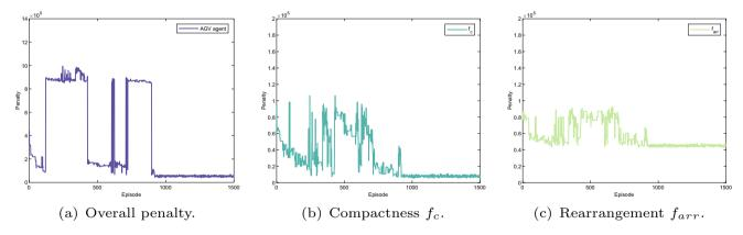
Fig. 19 Layout optimisation result (frame agent). The whole penalty regarding learning episode of the frame agent as shown in **a** consists of the penalty for compactness, rearrangement, production time and collision detection as indicated in **b**, **c**, Figs. 18e, and f, respectively
