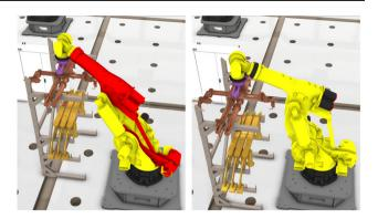
**Fig. 6** Joint limit triggered by relocation. In the left subfigure above, the robot third joint is out of the joint range. In contrast, for a different storage position in the right subfigure above, the robot third joint is in the joint range
