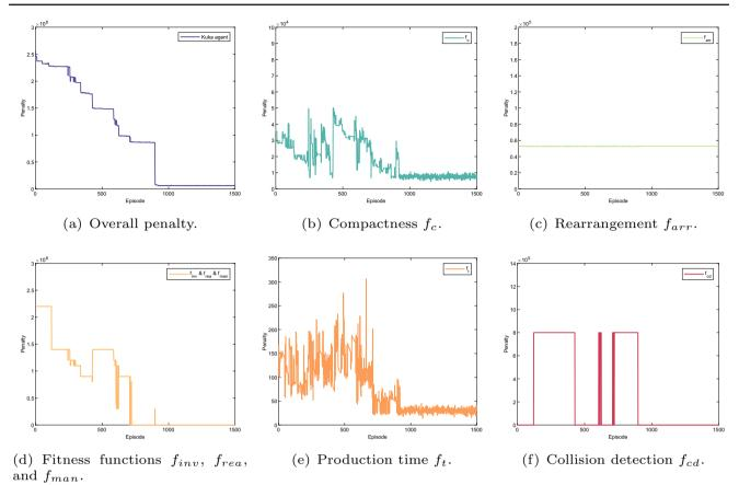
**Fig. 18** Layout optimisation result (KUKA agent). The overall penalty regarding learning episode of the KUKA agent as given in **a** is the sum of rhe penalty for compactness, rearrangement cost, robot configuration, production time and collision detection as presented in **b**–**f**, accordingly. Note that, the compactness penalty, rearrangement penalty
