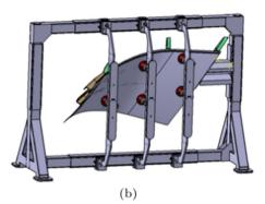
**Fig. 14** Frame for different product assembly. The designed frame aims to allocate different product assembly in a reconfigurable manner as shown in **a** and **b**. The vacuum cups located on the profile boards can be flexibly adjusted to hold different products
