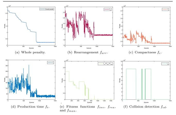
**Fig. 17** Layout optimisation result (all four agents). The sum of the rearrangement cost is given in Fig. 17b, including the rearrangement cost of each agent as presented in Figs. 18c, 19c, 20c, and 21c. The sum of the compactness cost is shown in Fig. 17c, consisting of the compactness cost of each agent as given in Figs. 18b, 19b, 20b, and 21b. The
