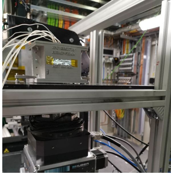
Figure 5.6 Assembled furnace at B16, Diamond Light Source.
