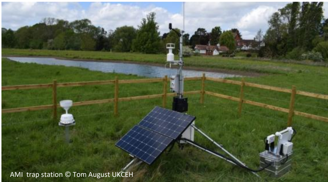
Figure 17. AMI trap station developed at UKCEH to monitor moths, birds and bats.
