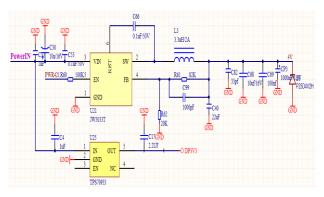
Fig. 11. The circuit diagram of a designed power-supply module used by D/RTUs.
