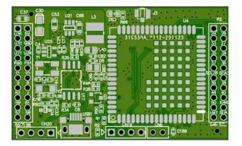
Fig. 12. The PCB layout of the developed MCU module's core board used by D/RTUs.
