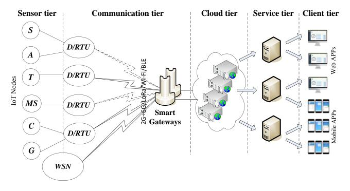
Fig. 3. The IoT multi-tier architecture of EMULSION.
