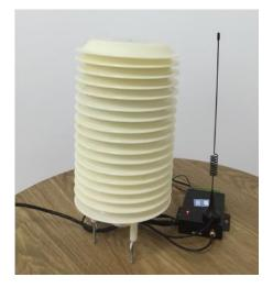
Fig. 6. A sample self-elaborated AQI monitoring station, utilized by EMULSION.
