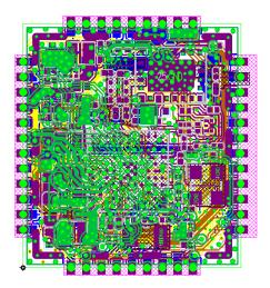
Fig. 13. The PCB layout of the developed MTK2503based GPRS module used by D/RTUs.
