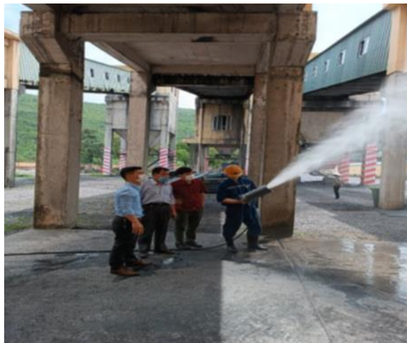
Fig. 1. Schematic diagram and test of the high-pressure water system with a full-cone nozzle (a) System of the high-pressure water ejector:
