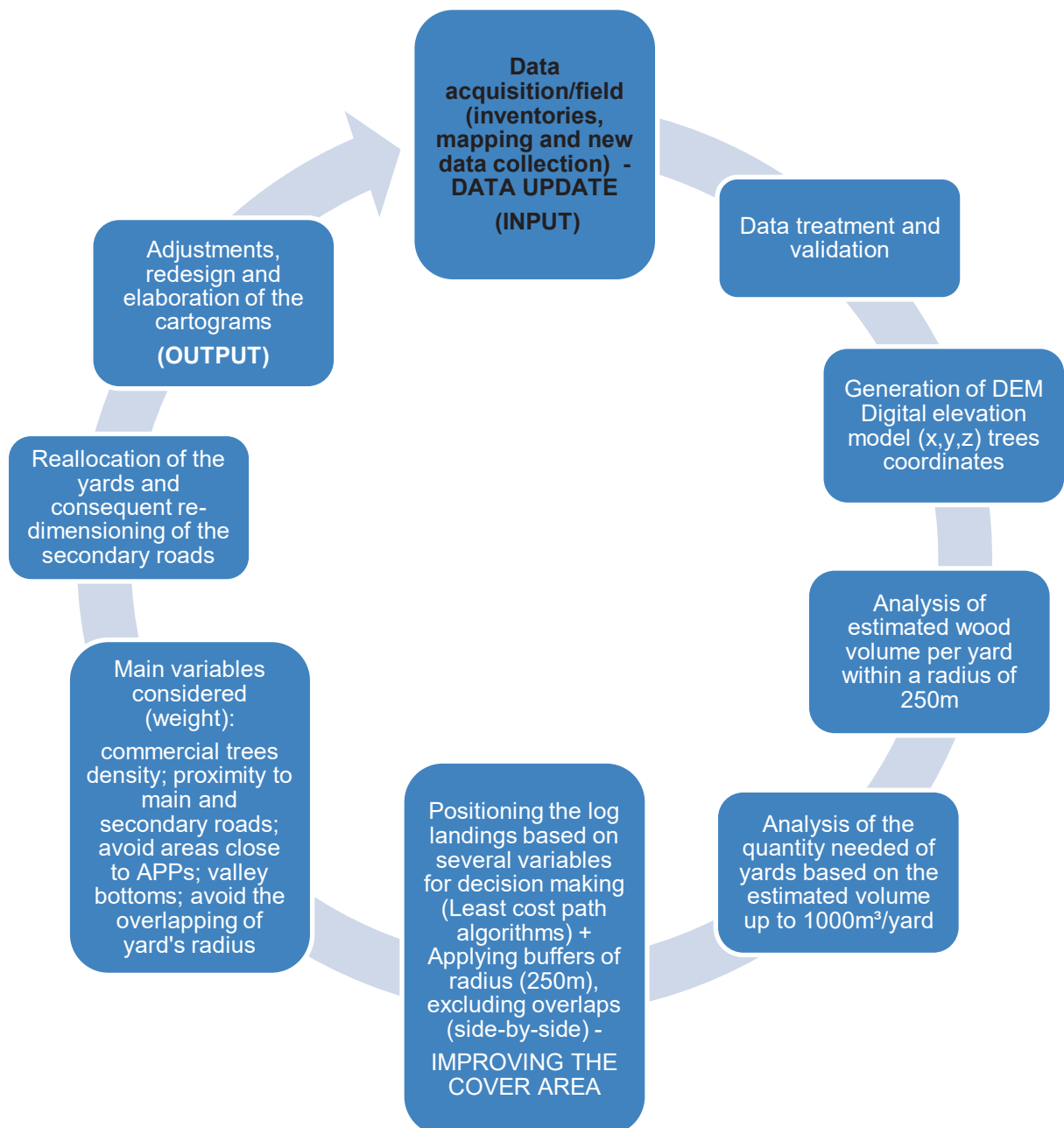
CHART 1 – FLOWCHART OF INFRASTRUCTURE IMPROVEMENT ANALYSIS, BASED ON PDCA PROCESS IMPROVEMENT TOOL.
