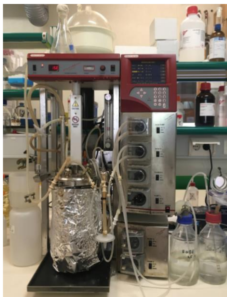
Figure 8 - Bioreactor used in C. cohnii fermentations.
