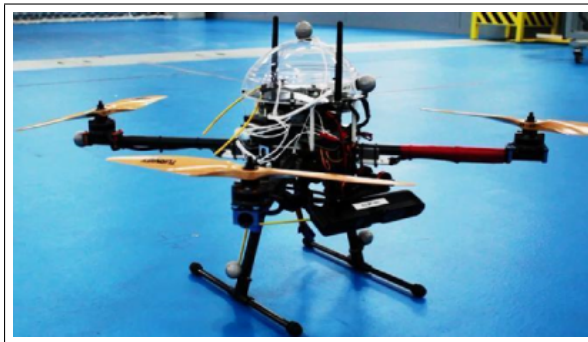
Fig. 9 UAS platform used for data acquisition. It was equipped with two RGB-D cameras Asus Xtion Pro Live, one facing forwards and another facing backwards.
