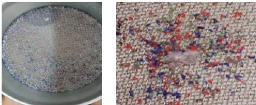
Figure 14. Fiber clumps with powder collected on a sieve (aperture = 1 mm).
