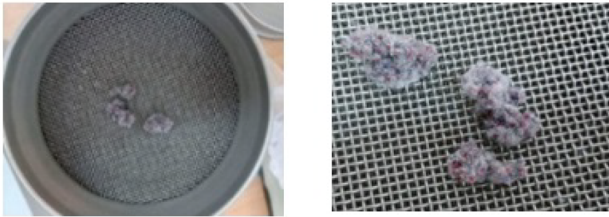
Figure 13. Fiber clumps collected on a sieve (aperture = 2 mm).
