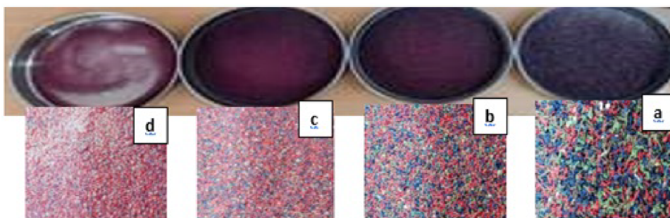
Figure 15. Retained powder with different aperture sizes: (a) 0.8 mm, (b) 0.6 mm, (c) 0.4 mm, (d) pan.
