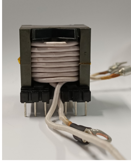
Figure 4.5: Physical realization of the transformer prototype.
