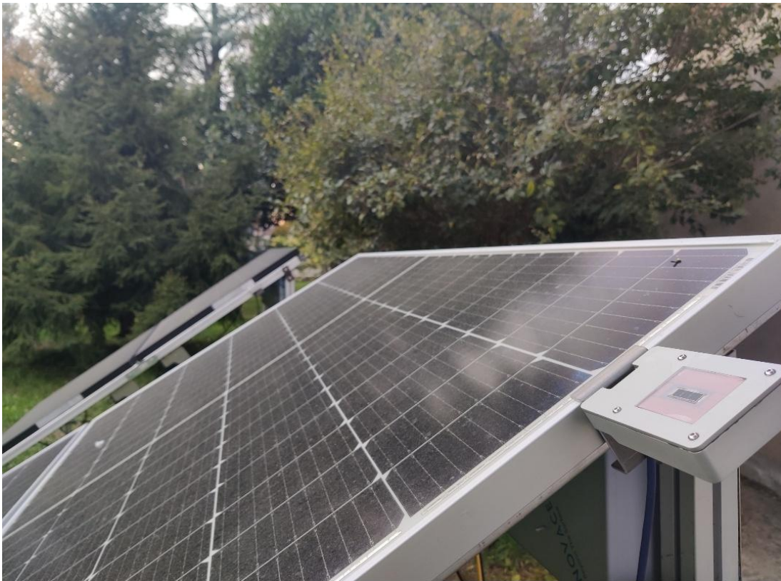
Figure 2.6 : Side view of the experimental setup with bifacial PV module and halfcut PV module with photovoltaic pyranometer attached to it
