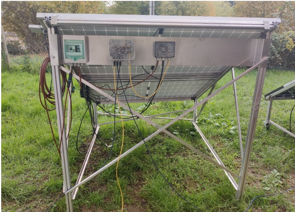
Figure 2.3 : Rear view of the experimental setup with the halfcut PV module
