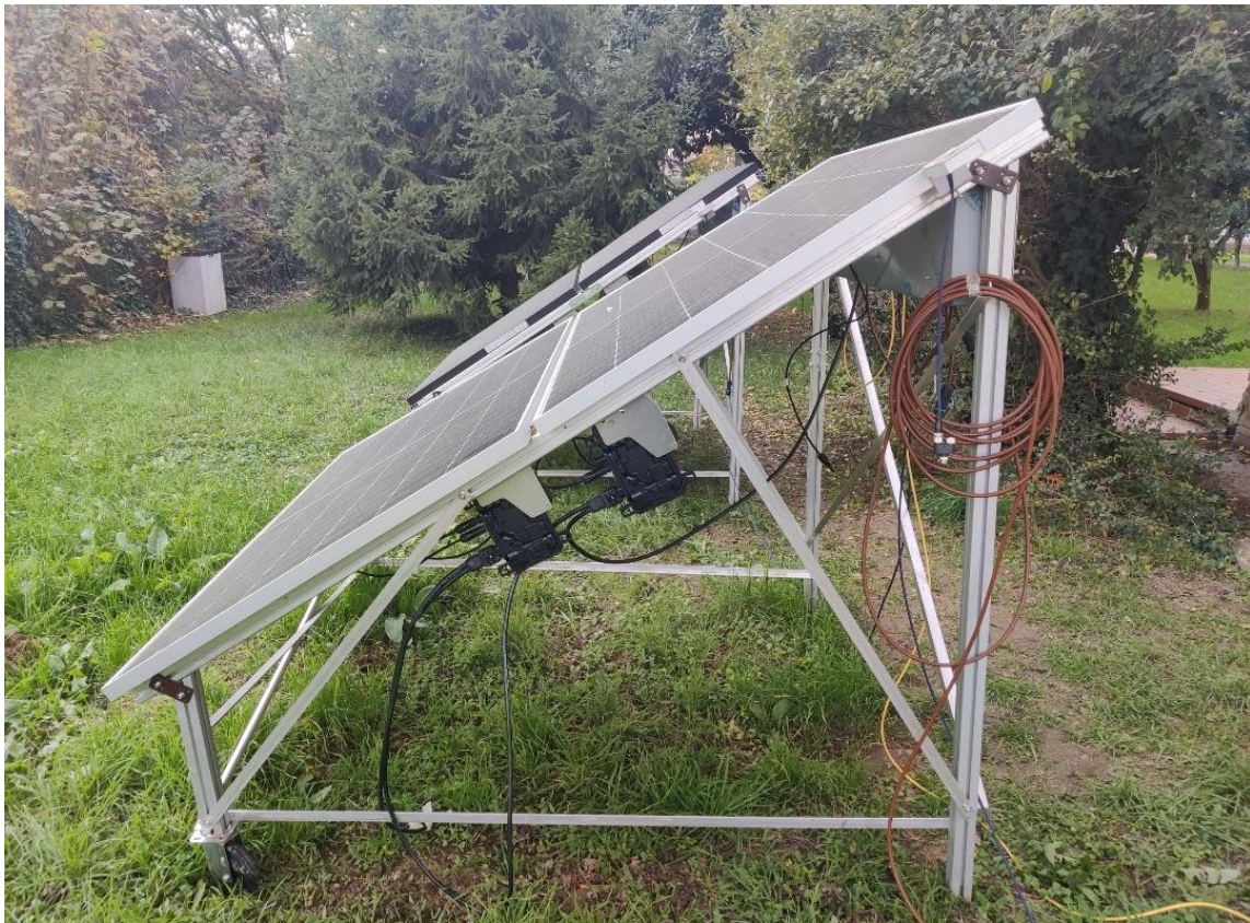
Figure 2.5 : Side view of the experimental setup with bifacial PV module and halfcut PV module
