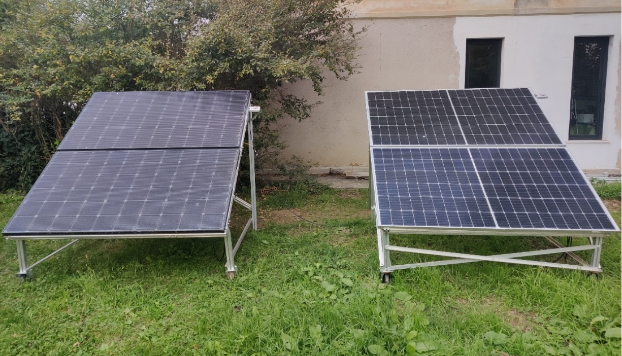
Figure 2.2 : Front view of the experimental setup with bifacial PV module on left and halfcut PV module on right
