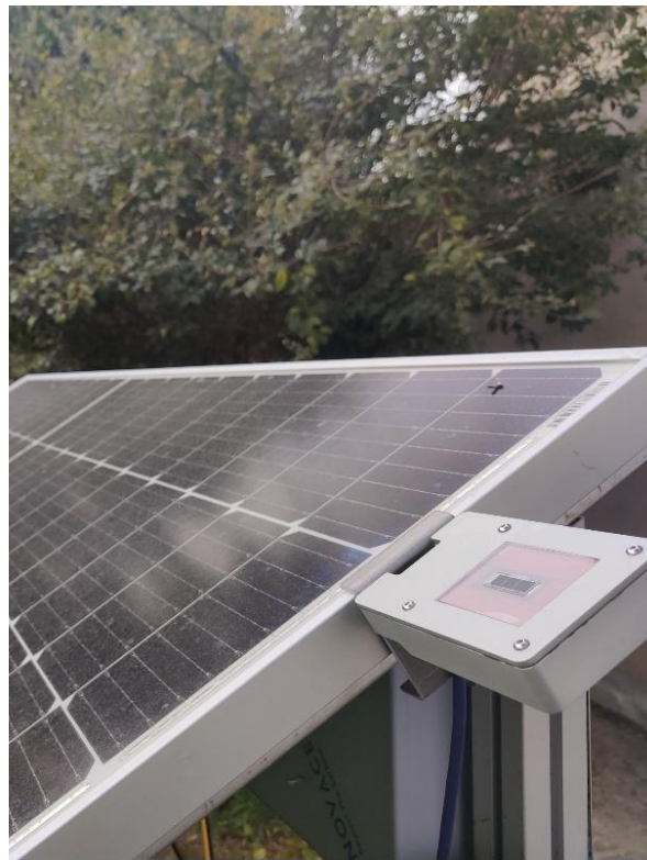
Figure 3.4 : Mounting of Sunmeter Pro photovoltaic pyranometer
