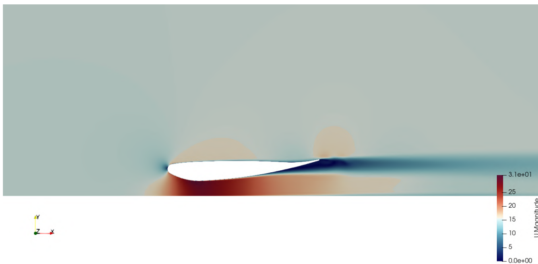
Figure 6.17: Velocity scene - 100 mm height
