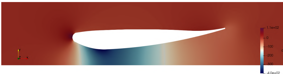
Figure 6.23: Pressure scene at peak C_l - first dynamic case
