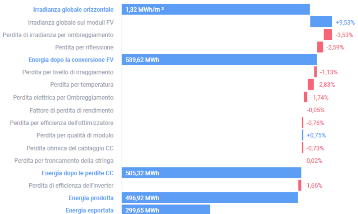
Figure 31: Diagram of the losses from Solar Edge Designer report (Appendix B)
