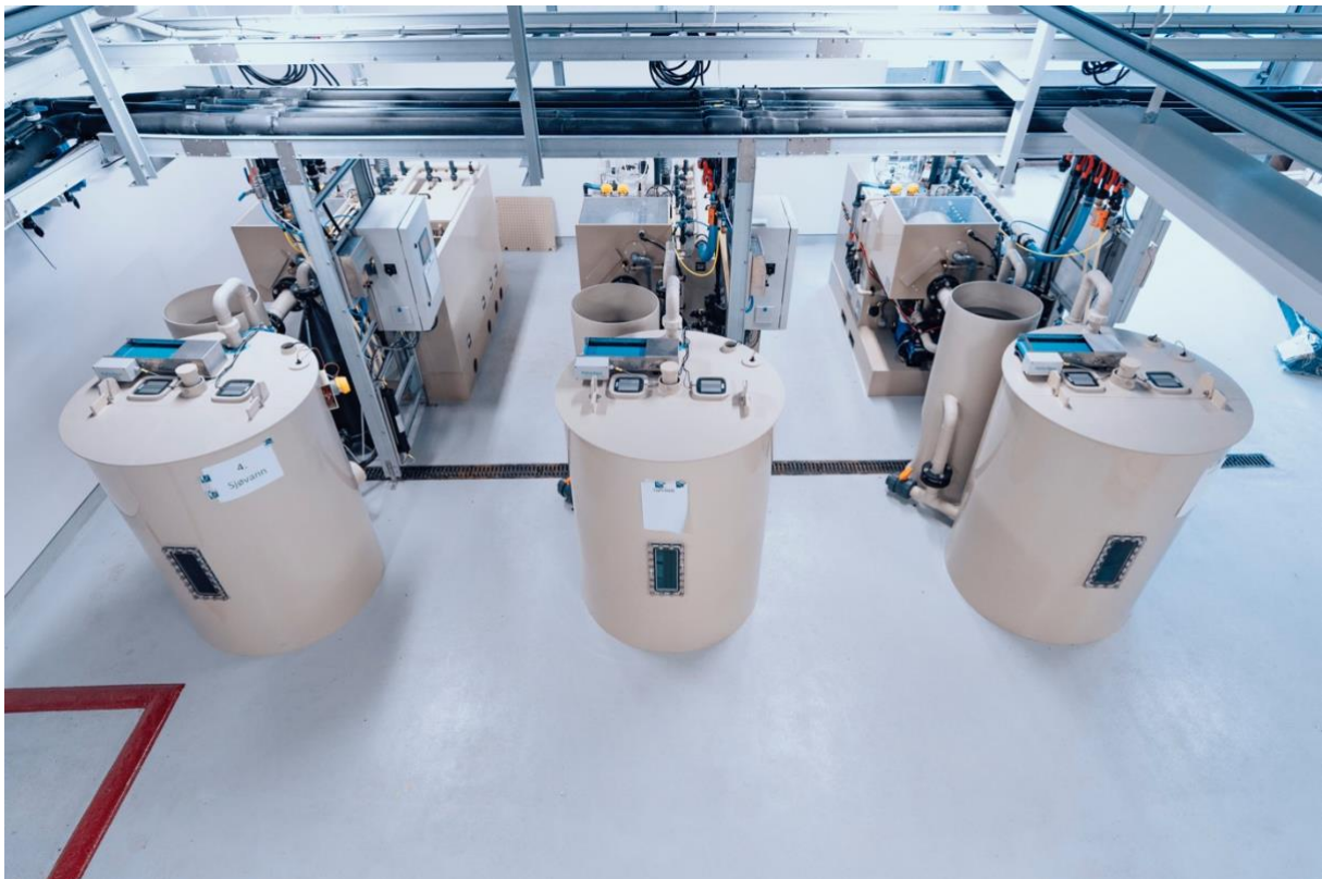
Figure 2.1: Picture of RASlab: Picture showing three separate RAS modules, with the rearing tanks in the forefront of the picture. Picture: (GC Rieber Eiendom, 2022).
