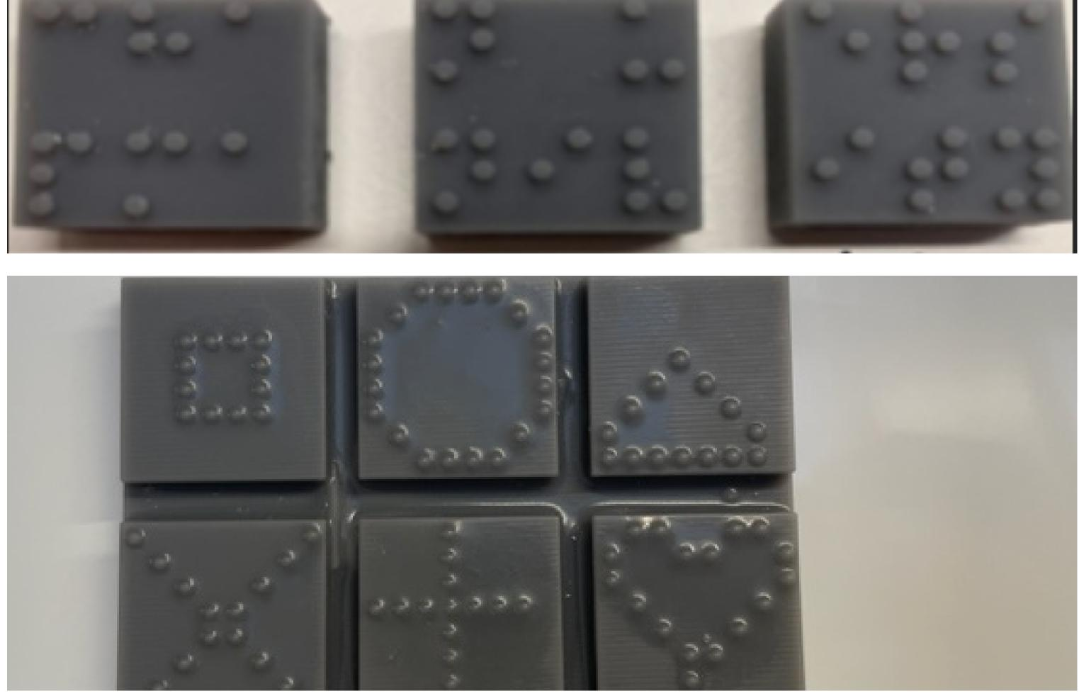
3D printed prototypes were created to test size, spacing, and pin configuration to find the optimum design for our refreshable braille display.
