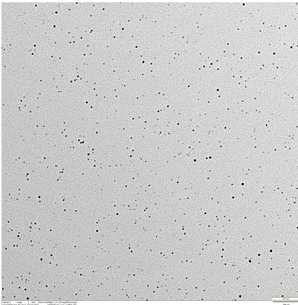
Figure S10 TEM image showing the deposited neutral Bi clusters after the splashing of the HNDs. This TEM grid was placed on the side (90 deg, G2) position 1.
