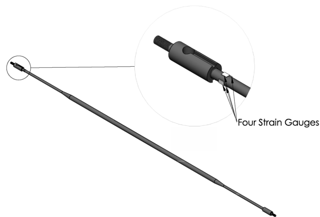
Figure 7. Schematic drawing showing the strain gauge installations on the flexible rod.
