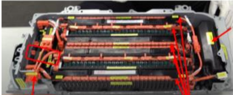
battery computer or BMS system under this plastic
