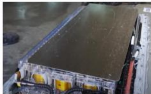
EM shield Sheet (electric magnetic shield) insulation
