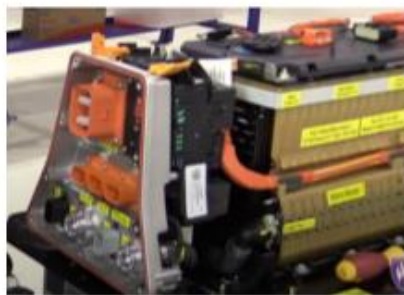
Battery contactor assembly is mounted by 2 studs
