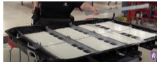
Remove module mounting bracket
