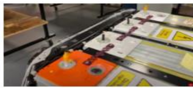
All bricks are connected in series
