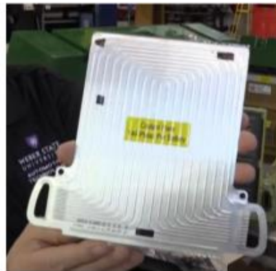
Plate is sandwich in-between the cells
