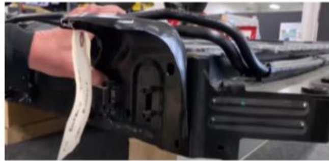
Front guide bracket during assembly
