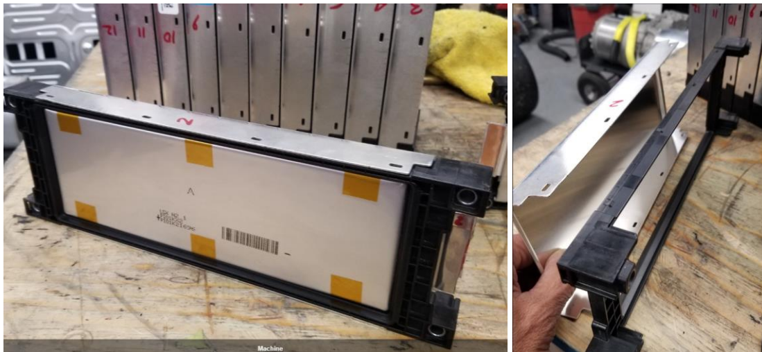
Figure 45. Heat Transfer plate in Module [61]
