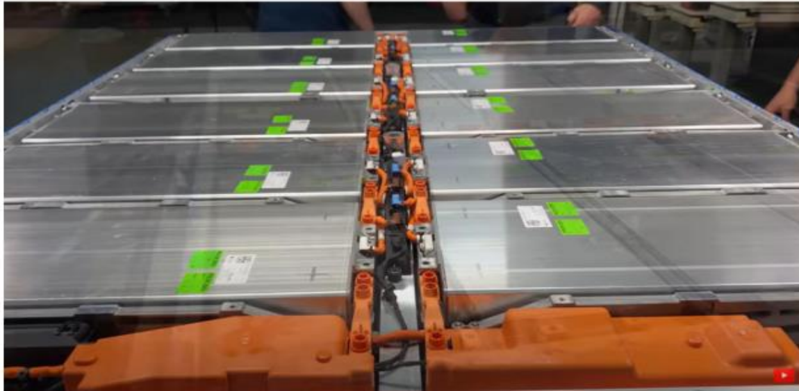
Spine design for the connectors
