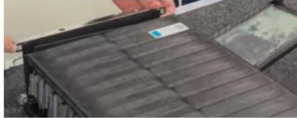
In end cap is self tapped which eliminate a need of extra nut (as chevy bolt) . 24 and 30 cells in battery
