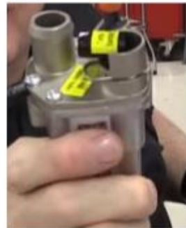
Coolant heater 1750 W
