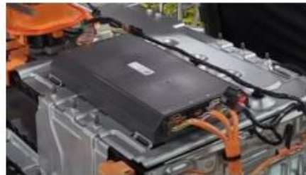
Disconnect BCM with all wire harness connection in specific order there are 6 connector
