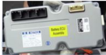
plastic cover mounted with 3 nuts under which there is BMS
