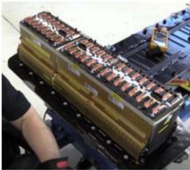
Two adjacent cell groups are welded together with copper bush bar
