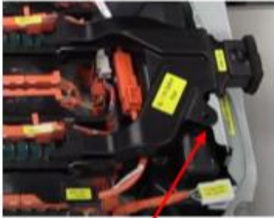
remove the duct by removing this 2 piece clip
