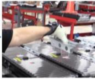
Disassemble module mounting bracket (6 bolt front 6 back and 3 on other side each)
