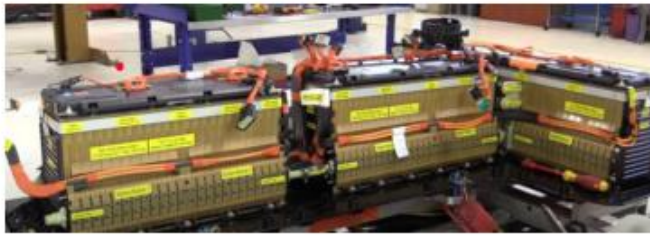
13 electrical connector Proper routing and groove for wire harness so that it should not rub on any thing and interfere with surrounding parts
