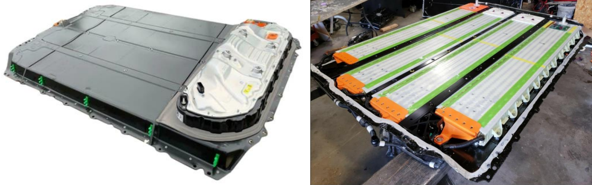
Figure 36. Tesla Model 3 battery pack[69]
