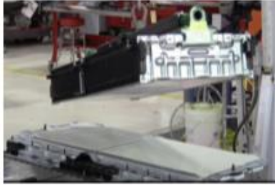
Disassemble upper Module
