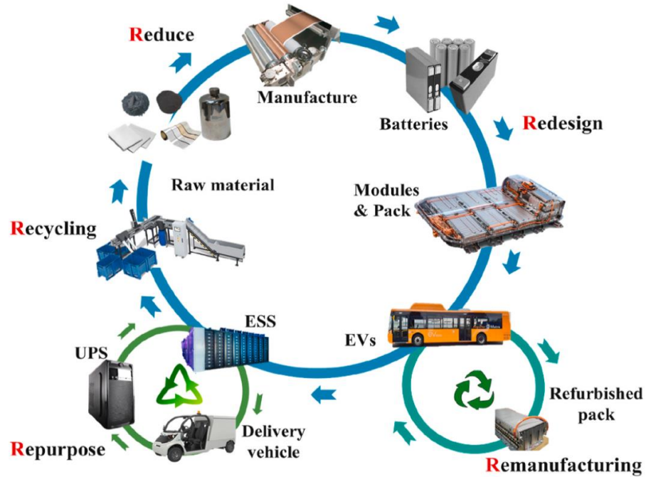
Figure 3. Circular value chain of retired lithium-ion batteries[10]
