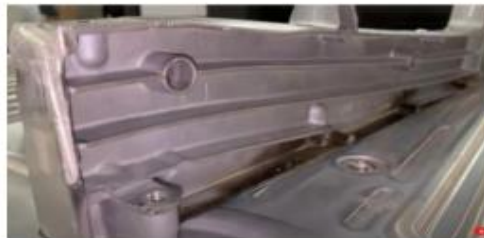
Casting and welding of cross members
