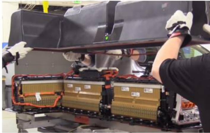
7 modules once upper cover is removed
