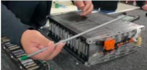
All cell are joined together with help of Long fasteners
