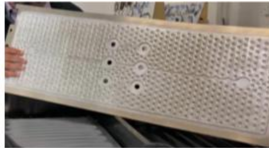
Back side of cooling plate is having dimple to make the flow of fluid turbulent so that it can absorb the more heat or excite transfer of heat and cold
