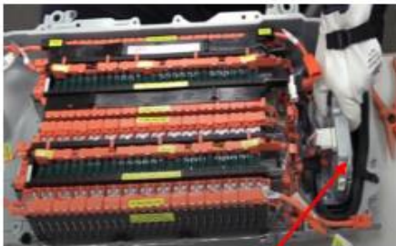
battery ECU unit is mounted by three nuts
