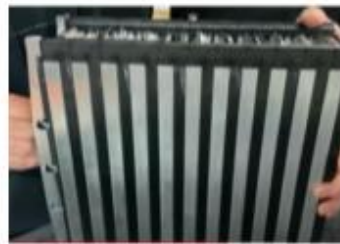
Aluminium plate is collecting the heat from the cell and transfer to the bottom which further transfer to cooling plate beneath it
