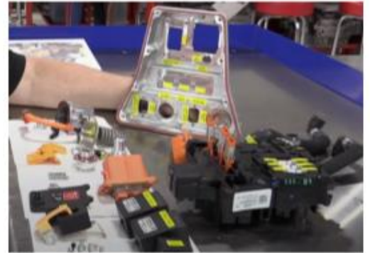
High voltage 2 terminal electrical connector, 4 bolt
