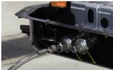
Put special connector with inlet valve and suck the coolant while creating vacuum and close the outlet valve to create the vacuum in cooling plates
