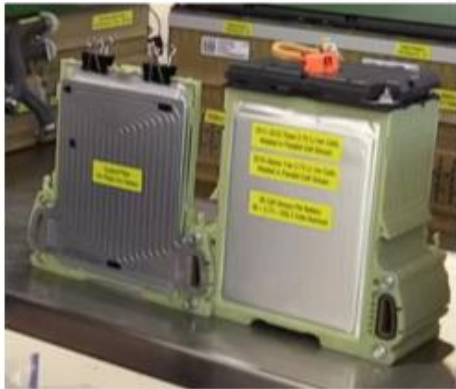
cell group of 2 or more cell in All cell groups are mounted together with help of long bolt on both side.
