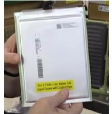
first generation - 3 cell are used in parallel in one group increase capacity without increasing the voltage 1 cell can give 55 amp per hour
