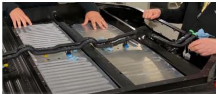
Two different size of cooling plates ,thermal interface compound which is in gray paste , helps in transferring the heat from battery module to the cooling plate
