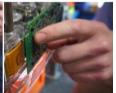
BMS is mounted with 2 rivets
