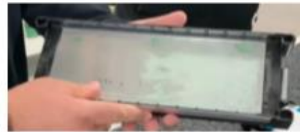
Aluminium plate with injection molded piece with aluminium
