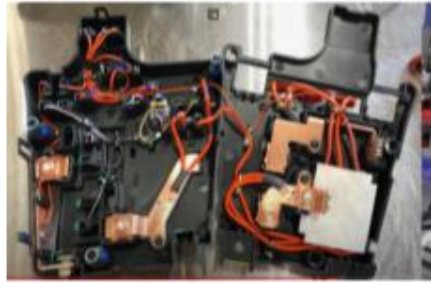
Contactor tray relay assembly
