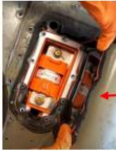
130 Amp fuse, mounted with 2 bolts
