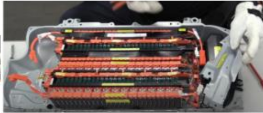
Remove metal cover from BMS
