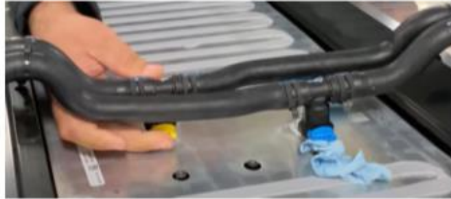
Quick connect to snap the cooling pipe in the place -10 quick connect
