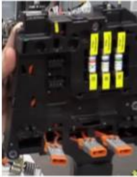
high voltage fuse
