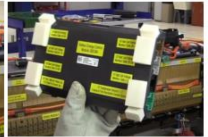
BMS: 8 electrical connectors : voltage sensing connecting except 2 7 and 8 low voltage -Temp sensor and current sensor in contactor assembly 8 communication line , GM land line, wake signal , ignition
