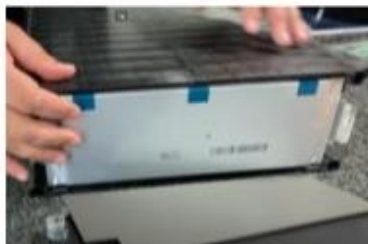
Foam to allow some expansion in pouch cell
