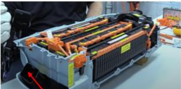
fan take the air from the cabin and blow it in the battery to keep it cool from this housing
