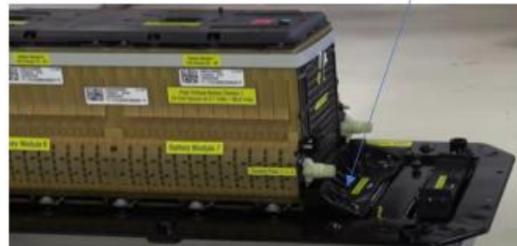
Front bracket to stop moving the battery in front mounted with 2 stud
