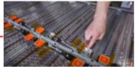
Each module is mounted with 2 bolts
