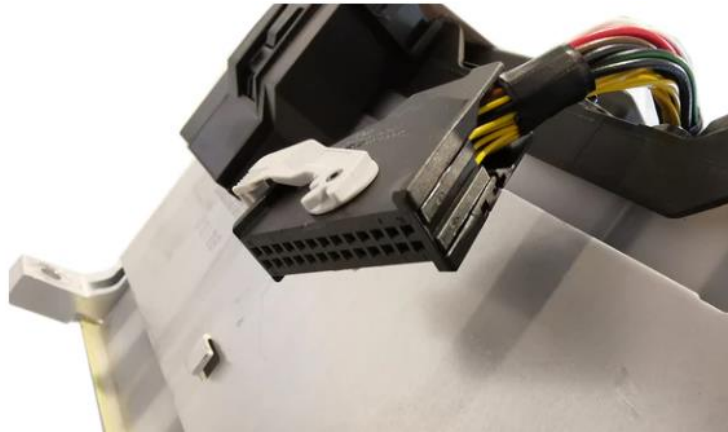
Figure 51. Connector of each module of BMW i3[77]
