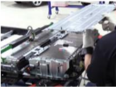
Disassemble bracket between section 4 and 5
