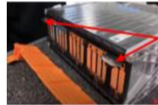
Terminals and protective cover in orange color
