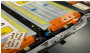
Jack nut with hexagonal head, holding the battery pack with lid
