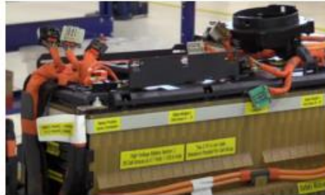
13 electrical connector Proper routing and groove for wire harness so that it should not rub on any thing and interfere with surrounding parts
