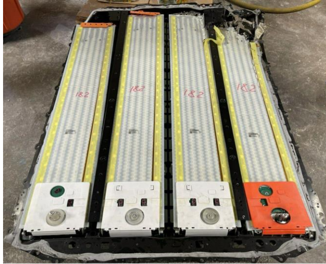
Figure 37. Module for Model 3[70]
