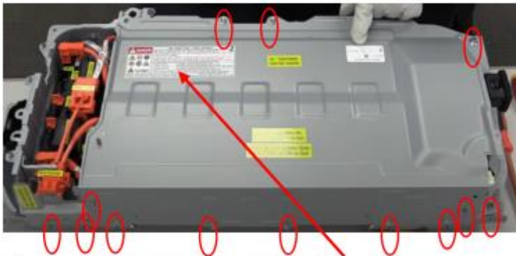
all nut and bolt are same except 2 bolt high voltage warning and phone no for battery recycling
