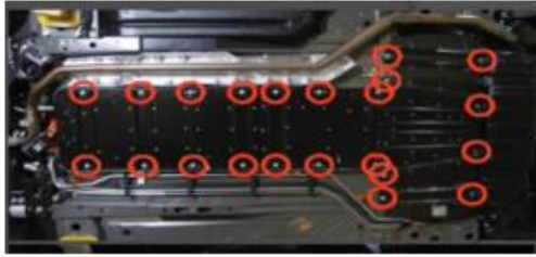
Battery pack Mounted at bottom with 22 bolts
