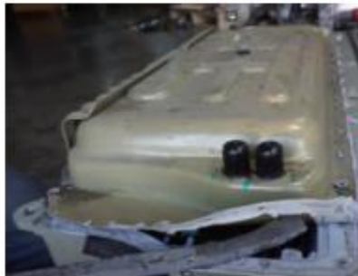
cover is mounted by 50 bolts approx. with sealant in middle
